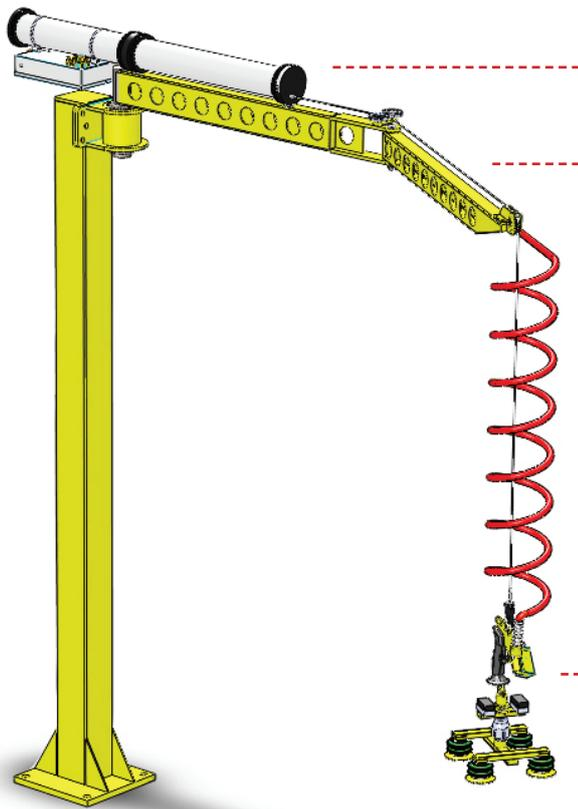
**Bal-Trol** - The small, flexible lifting cylinder is powered by compressed air only.
